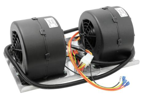
When replacing orignal 2 wire blower assembly with new 4 wire, high efficiency assembly you must bypass original resistor and connect wires (red, yellow, orange) directly to blower switch. New 4 wire motors have new style resistor built in to motor. Leave the (C) constant power & the (B) Battery terminal hooked up in their original locations on switch.
