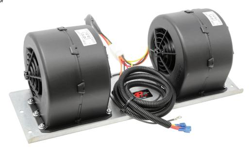
When replacing original 2 wire blower assembly with new 4 wire, high efficiency assembly you must bypass original resistor and connect wires (red, yellow, orange) directly to blower switch. New 4 wire motors have new style resistor built in to motor. Leave the (C) constant power & the (B) Battery terminal hooked up in their original locations on switch.
