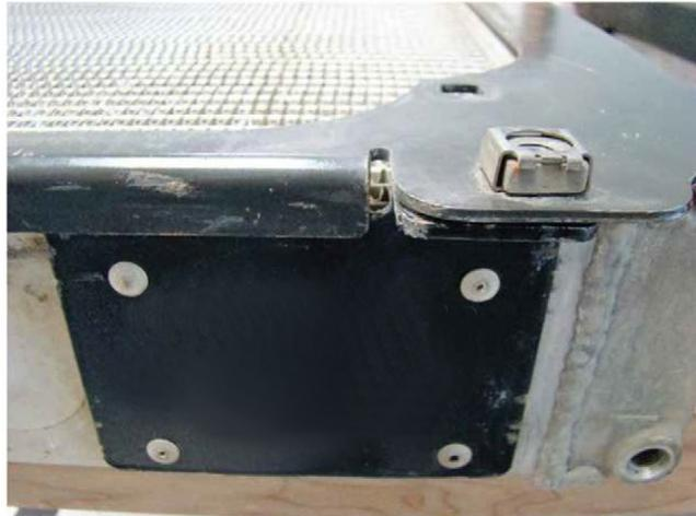
Old style radiator with bracket mounted to aluminum tank
