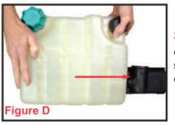
STEP 3: Lubricate the O rings with a small amount of coolant in the surge tank port. Slide the surge tank as shown in Figure D. Be sure that the O-rings are completely seated
