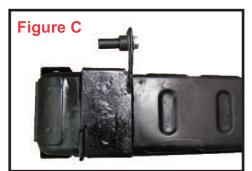
**STEP 2:** Position the small guide pegs as shown in Figure C.
