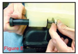
**STEP 4:** Insert the large peg and bolt into the surge tank and bracket as shown in Figure E. Tighten bolt carefully. Do not over tighten!
