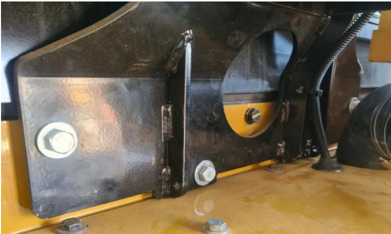
Fit supplied bracket & M10 bolts to OEM intake location on LH side of cabin.
