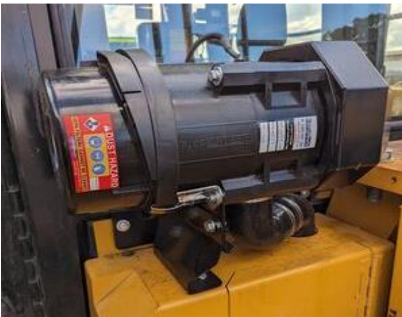
High pressure filtration unit installed
