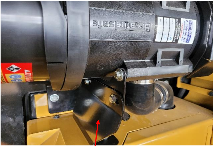
High pressure filtration unit installed inc. brace
